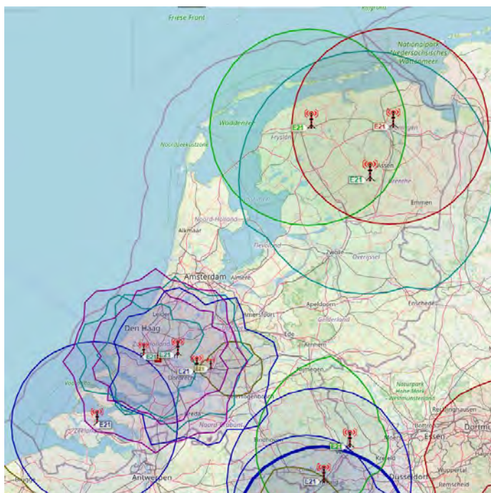
Figure 4: DVB-T2 coverage areas for channel 21 (source: fmScan.org)
